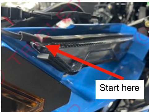
Using the longer strip clean the surface with alcohol and apply primer to the perimeter then apply led around the headlight.
