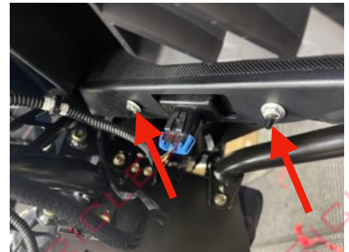
Using an 11MM socket unscrew the 2 metal retainer nut from the plastic studs and unplug the harness
